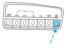
five seconds. After a successful reset, the message center will display OIL LIFE RESET TO 100%. (If you have established a personalized oil reset percentage, the display will show that percentage instead of 100%.) This reset procedure should be performed only after an oil change to ensure accurate oil life indications.
